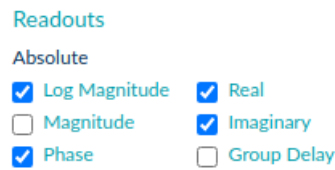
Figure 4.18: Select which readouts appear for a given marker. A marker will be visible on any trace type for which it has a readout enabled.
